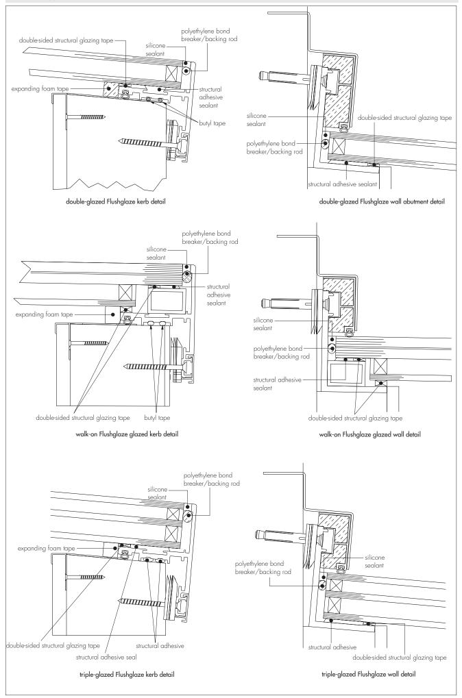
Figure 5 Typical fire-rated Flushglaze installation
